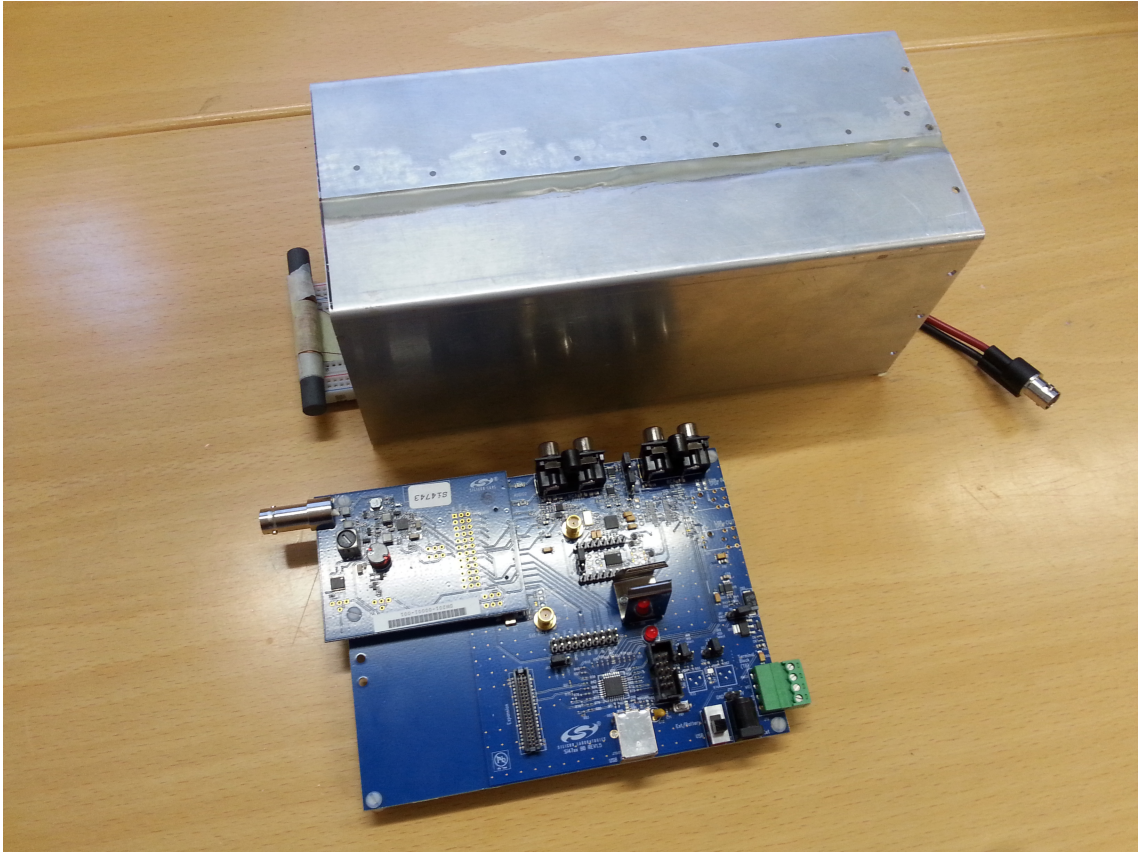
Figure 25: Prototype inside an aluminium body next to Si4743 development kit.
