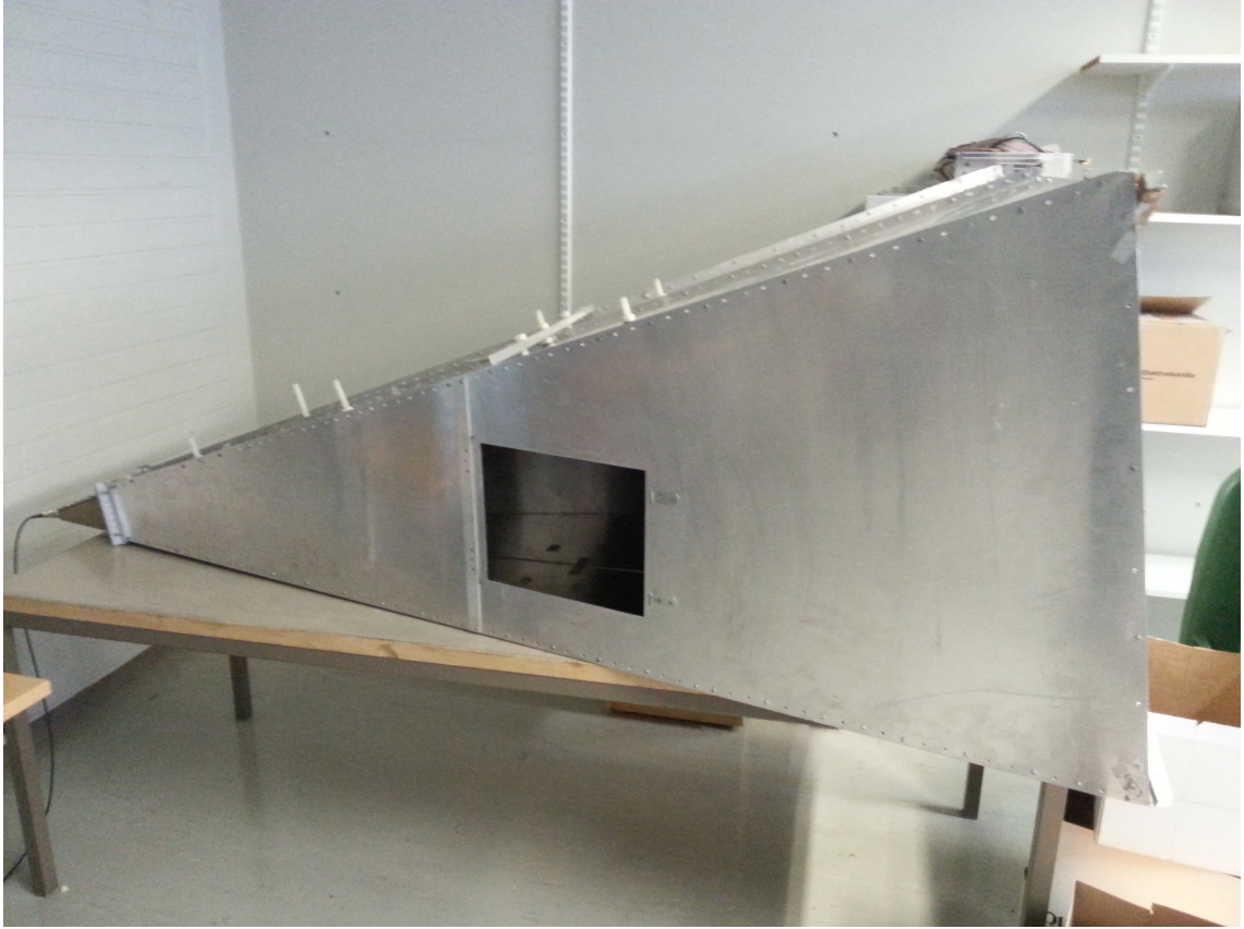
Figure 14: GTEM cell at Aalto University, Otakaari 5A, which was used in the measurements with the side panel removed. Photo taken by Petri Koskimaa.
